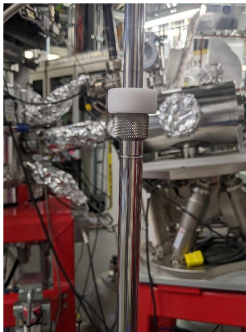
Transfer line seated and collar threaded onto dewar assembly
