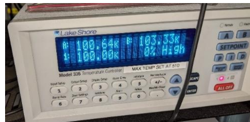
The front panel of the temperature controller, activated on range High, reading A, B, and setpoint 1 temperatures of ~100K, with 0% power flowing to the heater.
