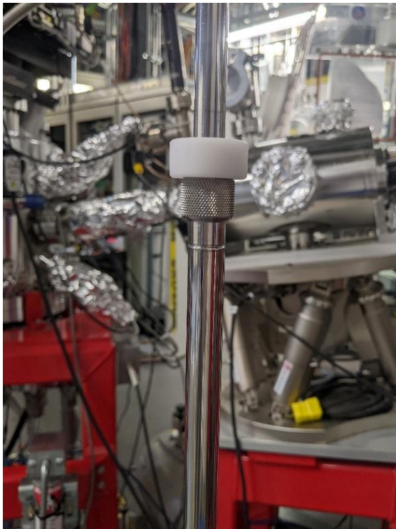
Loosen O-ring collar
