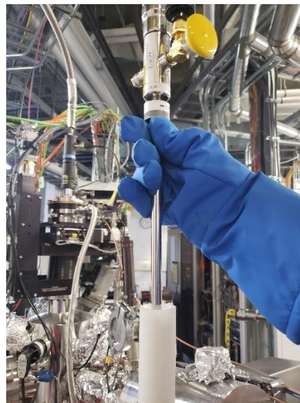
Dewar side of transfer line in white storage tube
