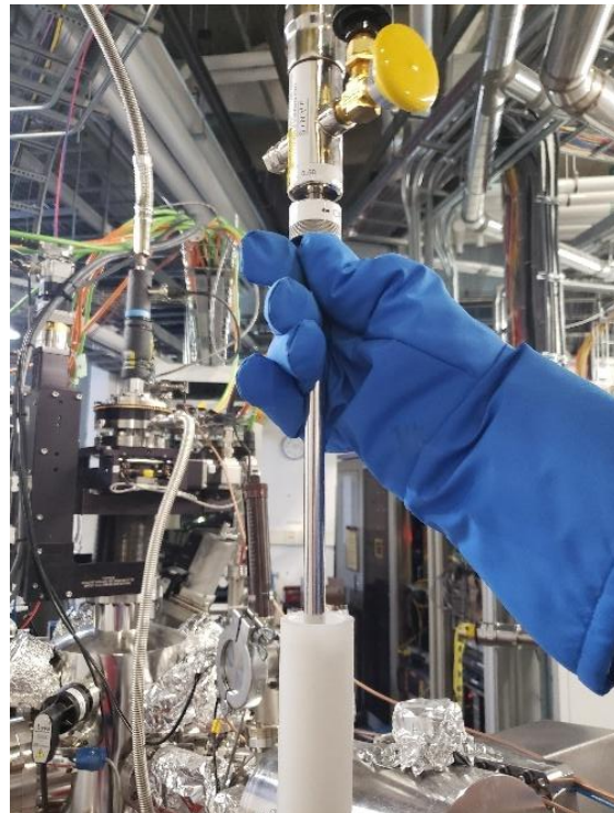
Transfer line moved back to storage
