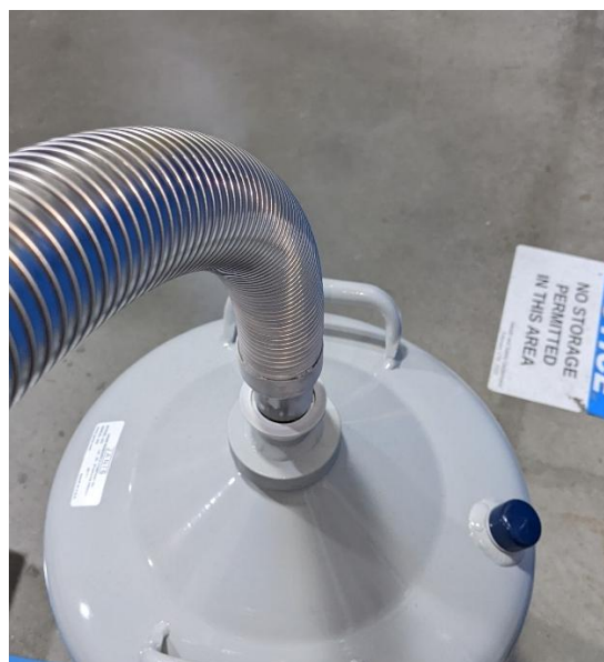
Insert non-pressurized fill hose into the neck of the dewar as shown.
