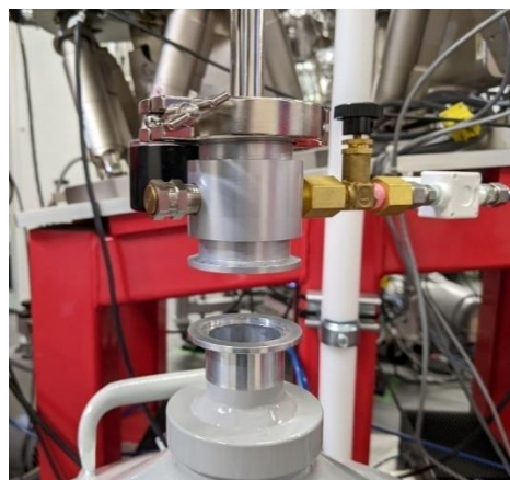
Assembly disconnected from dewar
