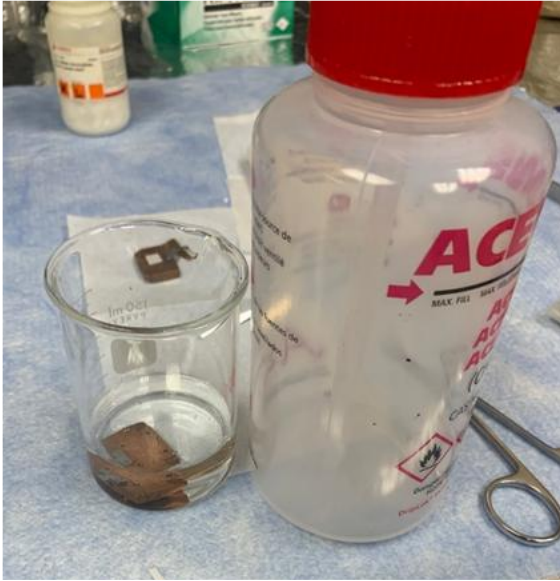
Picture 6: Beaker with an acetone fully submerged sample holder
