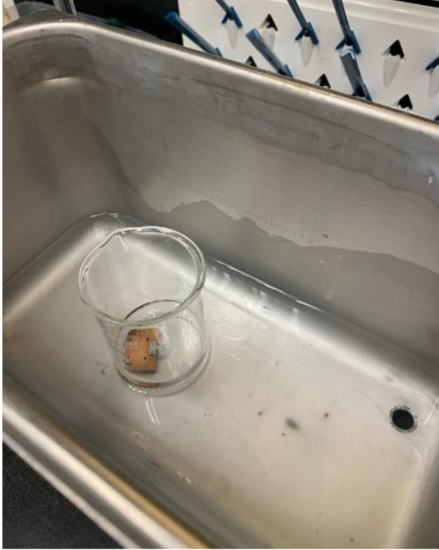
Picture 7: Ultrasonic cleaner with some water and the beaker containing the sample holder and the acetone
